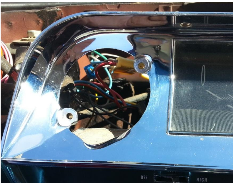
LEFT: Headlight switch bezel removed
